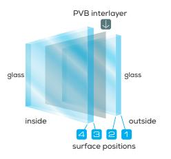
**INTERLAYERS** – Standard stocked laminated glass uses the same thickness and colour interlayer (generally 0.38mm thick). Only slight colour variation will occur as the overall glass thickness increases;
